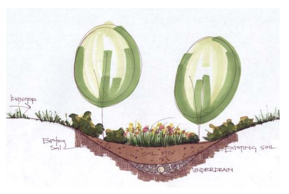
Section illustrating basic components of a raingarden
